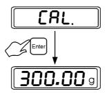
Please use , and , key to key in the mass values which you are going to calibrate, then press the key to confirm the value. When the display is flashing and showing the weight values, put the mass on scale. While scale is stable, the scale will return back to weighing mode. The calibration procedure is finished.
